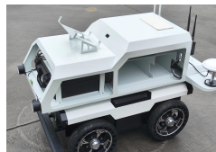
RTK-Enabled Autonomous Survey Vehicle for Topographic Mapping
